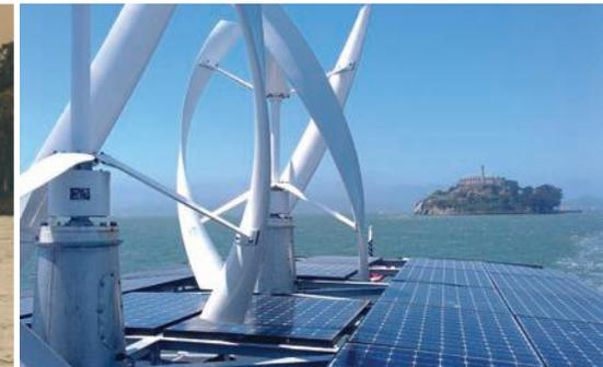
'The hybrid fleet uses power generated by ten-foot-tall wind turbines and photovoltaic solar arrays covering the awnings on the top decks.'
