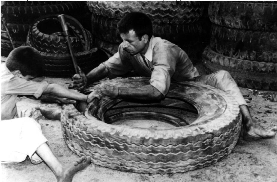
Figure 2: Manual Separation of the Tread from the Sidewalls, Karachi, Pakistan
